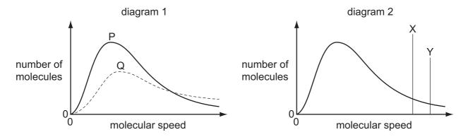
In diagram 1, one curve P or Q corresponds to a temperature higher than that of the other curve.
