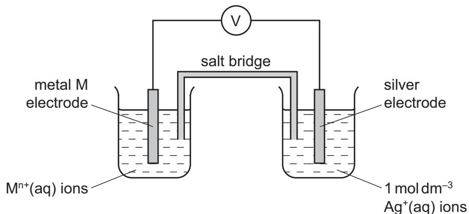
The metal electrodes of the two half-cells were connected via a voltmeter, reading to two decimal places. This was used to measure the cell potential of the cell.
