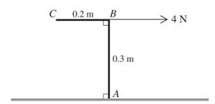
A uniform object ABC is formed from two rods AB and BC joined rigidly at right angles at B. The rod AB has length 0.3 m and the rod BC has length 0.2 m. The object rests with the end A on a rough horizontal surface and the rod AB vertical. The object is held in equilibrium by a horizontal force of magnitude 4 N applied at B and acting in the direction CB (see diagram).
