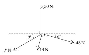
Coplanar forces of magnitudes 50 N, 48 N, 14 N and P N act at a point in the directions shown in the diagram. The system is in equilibrium. Given that  $\tan \alpha = \frac{7}{24}$ , find the values of P and  $\theta$ . [6]
