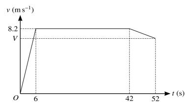
A sprinter runs a race of 400 m. His total time for running the race is 52 s. The diagram shows the velocity-time graph for the motion of the sprinter. He starts from rest and accelerates uniformly to a speed of  $8.2 \,\mathrm{m\,s^{-1}}$  in 6 s. The sprinter maintains a speed of  $8.2 \,\mathrm{m\,s^{-1}}$  for 36 s, and he then decelerates uniformly to a speed of  $V \,\mathrm{m\,s^{-1}}$  at the end of the race.
