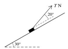
A block of mass 2.5 kg is placed on a plane which is inclined at an angle of  $30^{\circ}$  to the horizontal. The block is kept in equilibrium by a light string making an angle of  $20^{\circ}$  above a line of greatest slope. The tension in the string is T N, as shown in the diagram. The coefficient of friction between the block and plane is  $\frac{1}{4}$ . The block is in limiting equilibrium and is about to move up the plane. Find the value of T.
