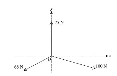
Three coplanar forces of magnitudes 68 N, 75 N and 100 N act at an origin O, as shown in the diagram. The components of the three forces in the positive *x*-direction are -60 N, 0 N and 96 N, respectively. Find
