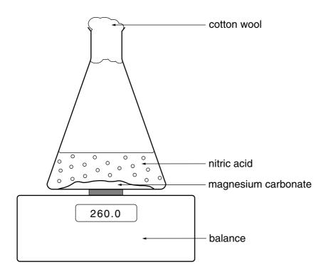
The flask was placed on a balance and the mass of the flask and contents recorded every minute. The results are shown in the table.
