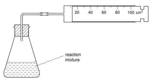
The volume of hydrogen collected at one minute intervals was measured. Use the diagrams to record the volumes in the table.
