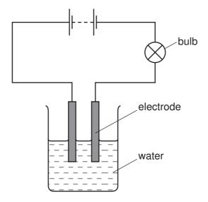
After the student adds substance  $\mathbf{X}$  to the water, the bulb lights.
