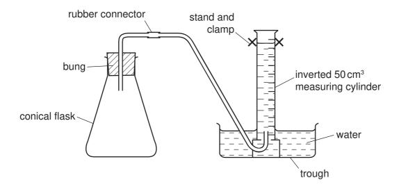
Remove the bung from the conical flask and move the measuring cylinder away from the delivery tube without letting any water run out. Twist one of the strips of magnesium provided to break it into four pieces and place all of them into the conical flask.
