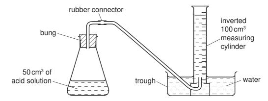
Using a measuring cylinder, 50 cm³ of acid **X** was poured into the conical flask. 0.5 g of magnesium ribbon was added to the conical flask and the bung replaced.
