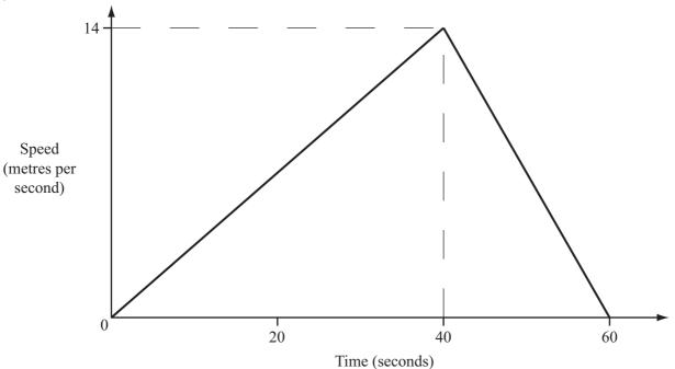
The diagram shows the speed-time graph of a bus journey between two bus stops.
