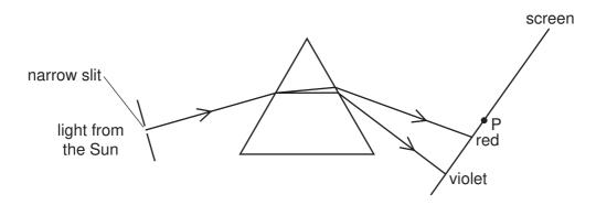
A thermometer placed at P shows a large temperature rise.
