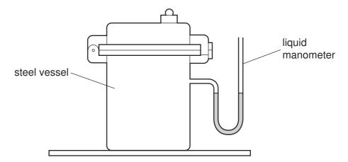
What value does the liquid manometer give for the pressure in the vessel?
