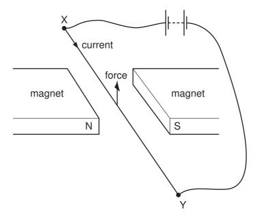
If the north and south poles of the magnet exchange positions, in which direction will the force on the wire act?
