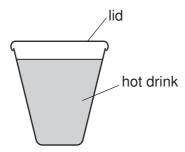
When the lid is removed, the rate of heat loss from the drink increases.
