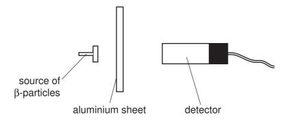
Eventually a sheet which is 2.0 cm thick is used. The reading on the detector decreases, but does not fall to zero.
