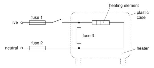
Which of the fuses are correctly placed?
