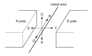
In which direction or directions must the wire be moved to induce an e.m.f. across the ends of the wire?
