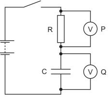
What happens to the reading on the voltmeter Q and what happens to the energy stored in the capacitor?
