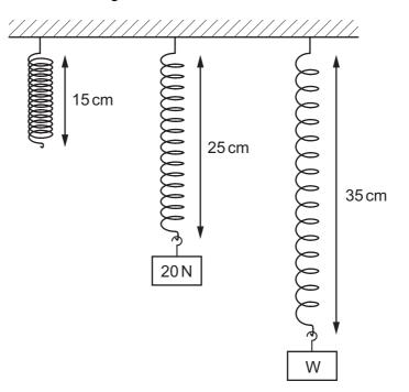
The extension of the spring is directly proportional to the weight hung from it.
