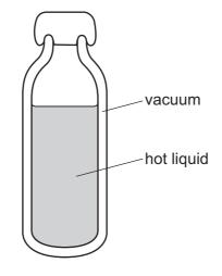
How does thermal energy pass through the vacuum?
