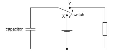
The switch can be moved between position X and position Y.
