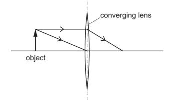
An image of the object is formed on a screen to the right of the lens.
