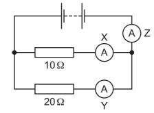
Which ammeter has the largest reading?
