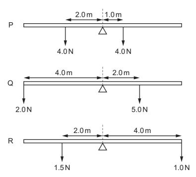
Which beams rotate clockwise?
