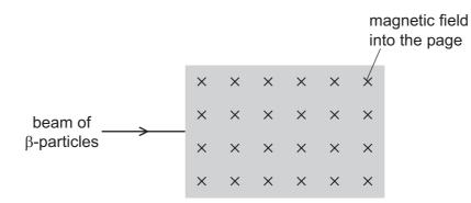
In which direction is the beam of  $\beta$ -particles deflected as they enter the magnetic field?
