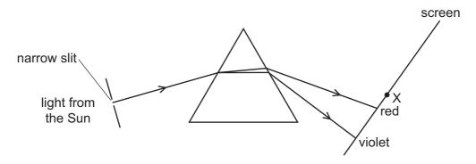
A thermometer placed at X shows a large temperature increase.
